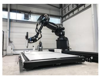
significantly decreases the amount of waste during the production of a part. CEAD robot extruders can process virtually all fiber reinforced thermoplastic materials and thus the end part can have the desired mechanical properties for its purpose. The technology is therefore widely applicable to many industries. Thermoplastics can be recycled after the end of the product life cycle and can be reprocessed multiple times, decreasing the environmental footprint.
